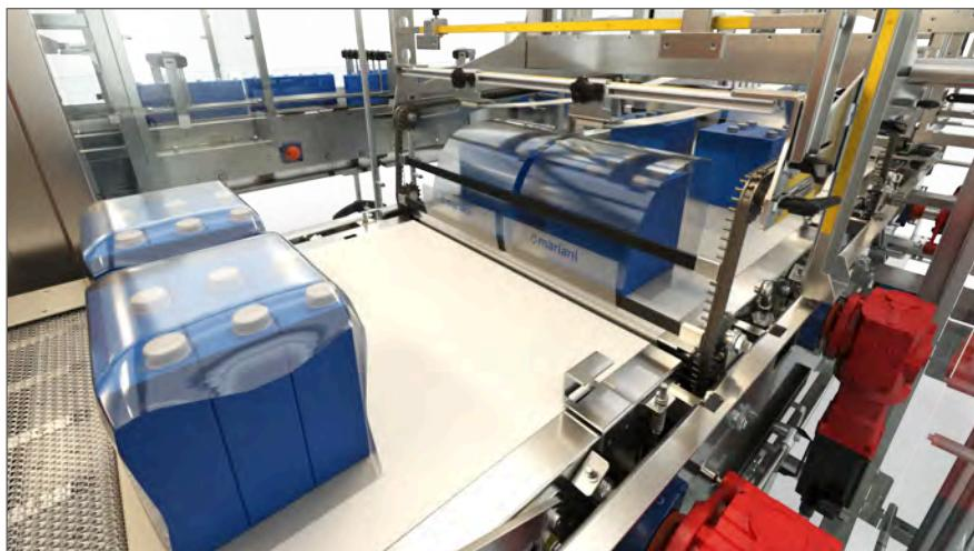
The machine employs a proven design concept at the infeed for product handling and bundle forming, producing tightly wrapped square packs which guarantee cartons' integrity and safe handling.
