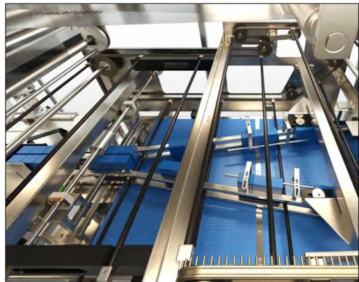
Packs, during the feeding cycle, are wrapped in film before they enter the shrink-tunnel resulting in a tightly wrapped final bundle. This operation is done by a cut and seal unit that ensure the perfect closure of the bundles.
