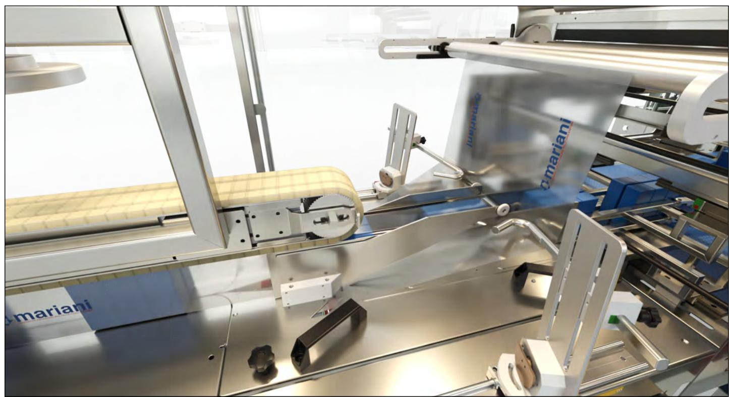
Pre-grouping packs gets into the film cover section; in this stage packs are fully wrapped and sealed at the bottom.
