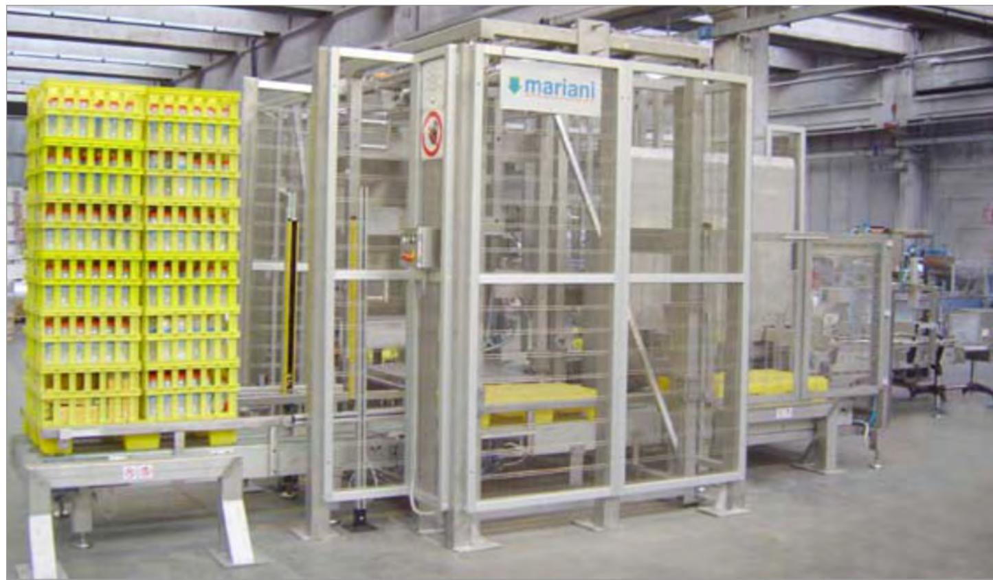
Machine designed to palletise stacks of plastic crates or metal buckets mod. **PMP 465**
