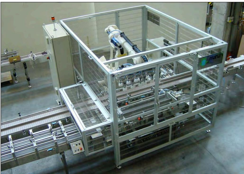
The operating area and the carrying capacity make this robot particularly suitable for handling small packages grouped
