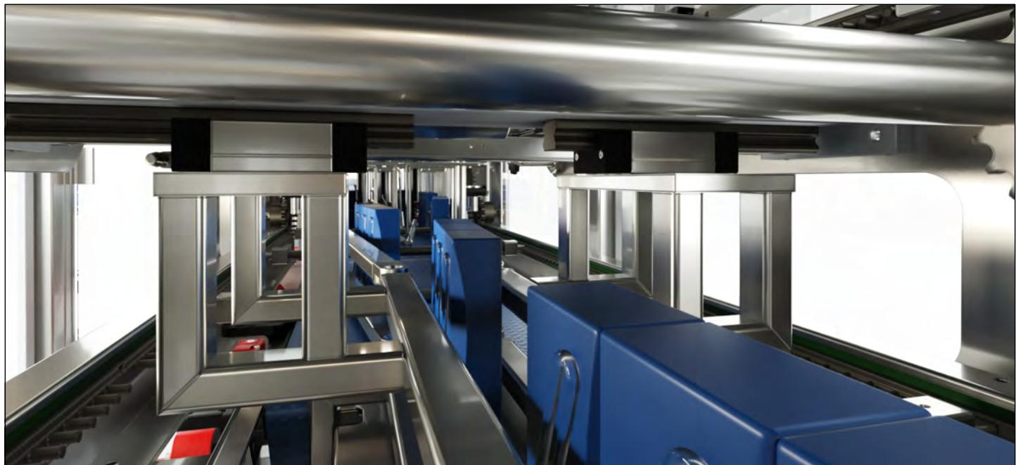
Products arriving on the in-feed conveyor are arranged and laned by means of special parallel belts at machine's entry, distributed into one or two rows and grouped according to the required formats to be packed.
